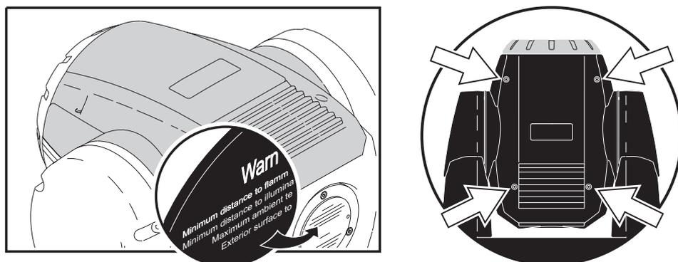
**Figure 6: Identifying and removing the upper head cover**
