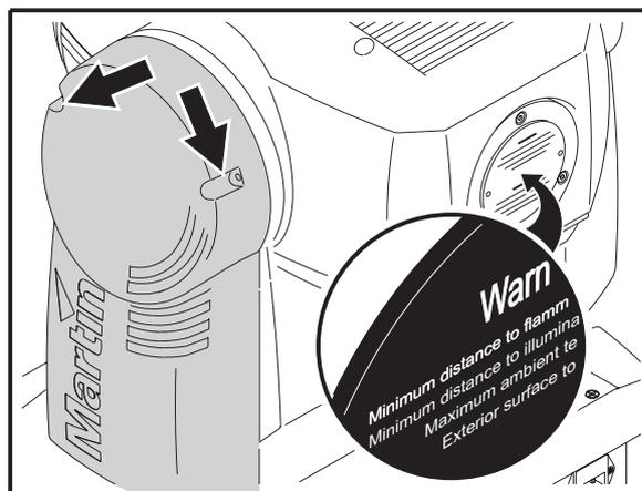
**Figure 16: Identifying and removing the left-hand yoke cover**
